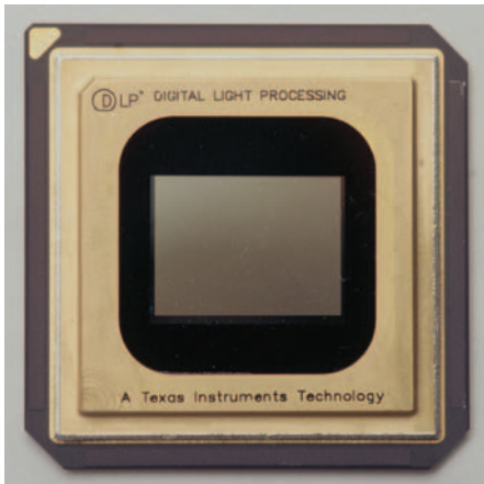
Figure 3: XGA resolution DMD (1024 x 768 pixels) as used e.g. for beamers
