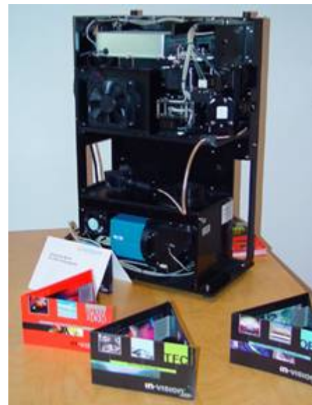
In-Vision Digital Imaging demonstrated a complete DLP light engine built into a biotechnical DNA sequencer
